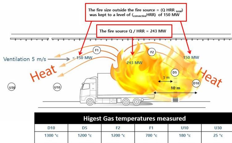
Fig. 5 – Full scale tunnel fire test (Free burn) – Spain 2018<sub>2</sub>)
